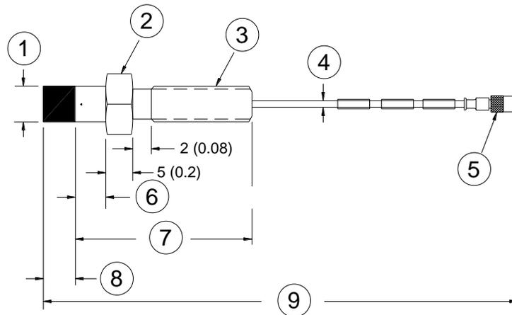
1. Probe tip, 8.0 mm (0.31 in) diameter
