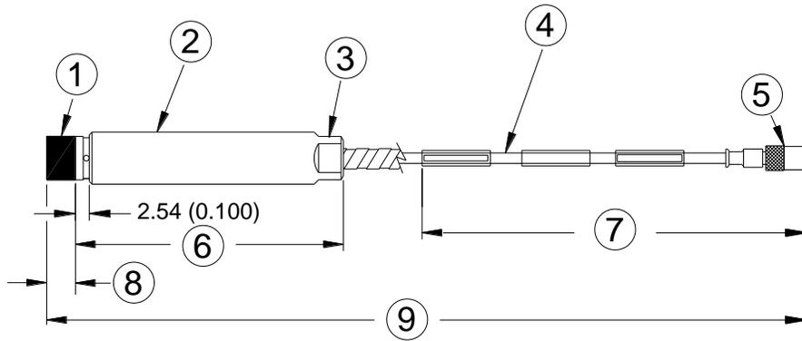
1. Probe tip, 8 mm (0.31 in) diameter
