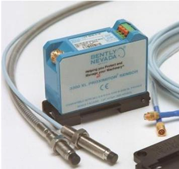
The system provides an output voltage that is directly proportional to the distance between the probe tip and the observed conductive surface and can measure both static (position) and dynamic (vibration) values. The system's primary applications are vibration and position measurements on fluid-film bearing machines, as well as Keyphasor\* reference and speed measurements<sup>3</sup>.
